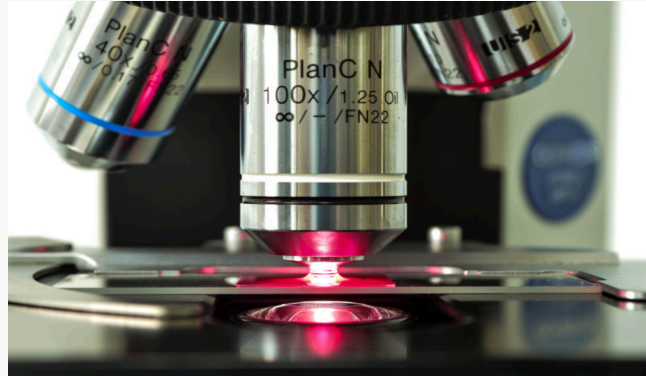
Figure 1: Oil / Water immersion microscopy setup.
