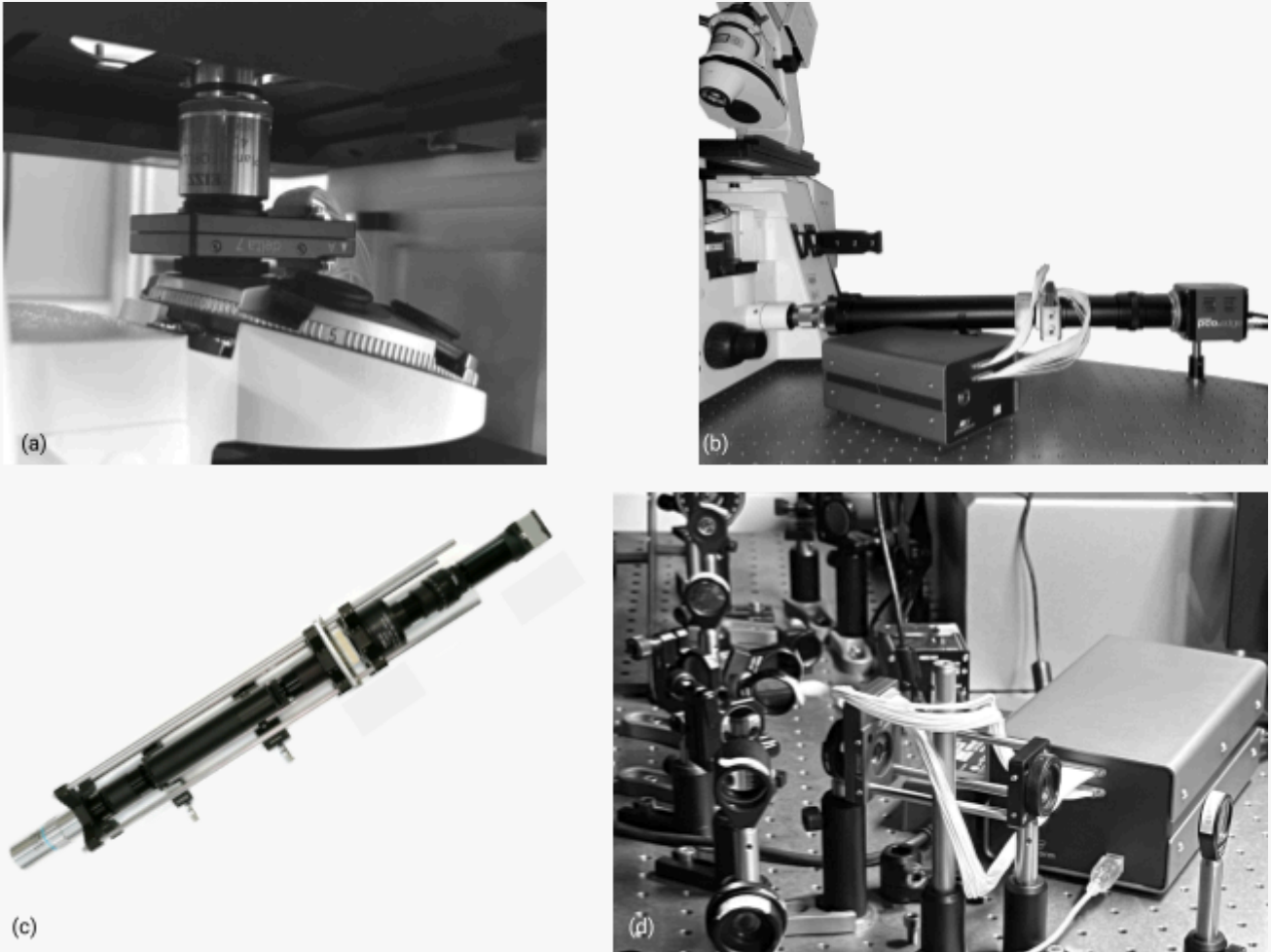
Figure 5: Examples of DPP-based AO systems in commercial and custom-built microscopes. (a) DPP between the objective and turret in a commercial microscope. (b) DPP at the conjugate pupil plane of a commercial microscope (via relay optic). (c) "World's smallest AO microscope" for fluorescence wide-field imaging [5]. (d) DPP in the illumination path of a custom-built two-photon microscope (collab. with Prof. Alexander Jesacher, Medical University of Innsbruck).
