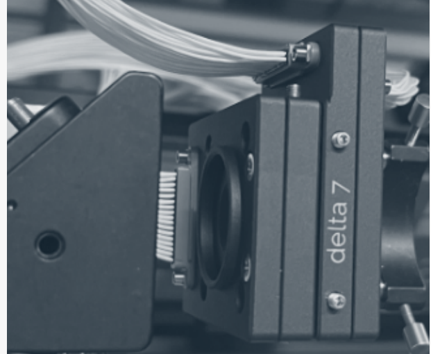
Figure 6: Cascaded DPPs in the form of two stacked Delta 7.
